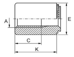
Female thread A = M4Height K = 18Min distance to edge = 4.0Outer diameter E = 8Plate thickness = from 2.4Recommended bore diameter +0.05 = 5.00Thread length = 8.0
